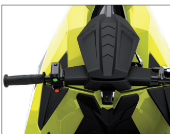
Ergal handlebar with co-molded grips and large soft pad
